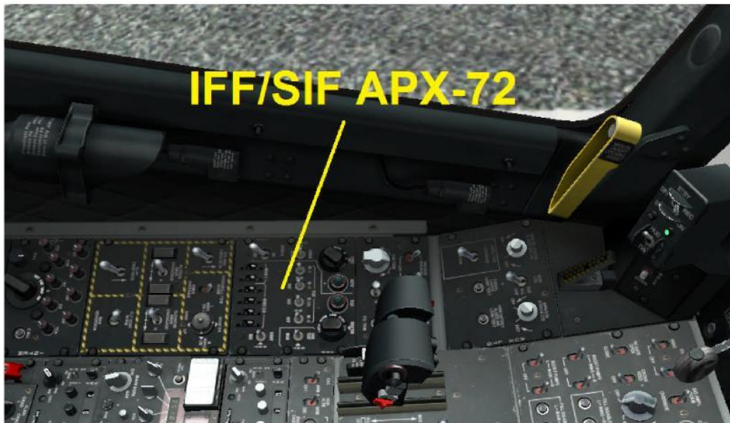
Figure 21A-10C IFF/SIF control panel
