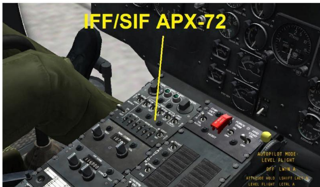
Figure 22UH-1 IFF/SIF control panel
